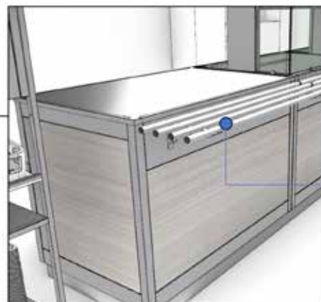
Optional 7/300 Scorriavassoio richiudibile in tubo INOX Foldable stainless steel tubular tray slider
